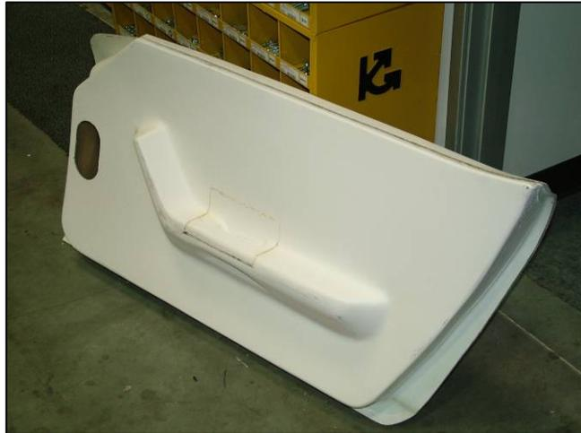
These Z doors are designed to fit on 1970-1978 Datsun Z. There is no hardware included with the doors. They are designed to be attached either semi-
