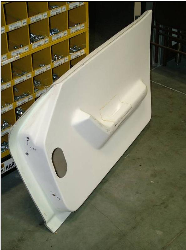
For attaching the doors to hinges, you'll have drill holes for hinge bolts in the locations indicated by scribe marks in the gel coat in the front door jamb area. You'll then have to cut out holes in the inner panel (if you get the doors with the full inner panel), and reach through into the inside of the door jamb area to insert metric-thread bolts (you can re-use the stock bolts) through the fiberglass into the stock hinges.
